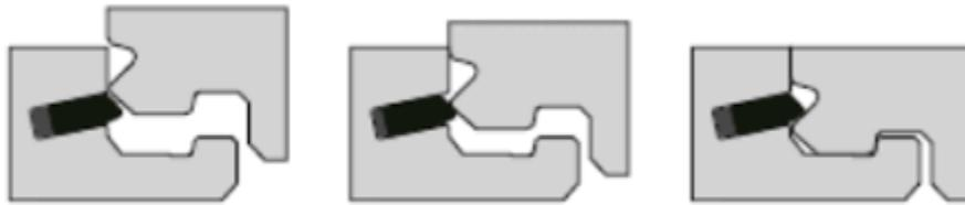
Shocks caused by transporting the boxes could cause the tongue to move and it could come out of its groove. Simply push the tongue back into place and install the board as explained below.
